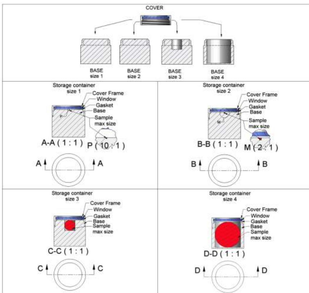
**Figure 2.** Possible design of the internal sample holder (courtesy Kayser Italia).
