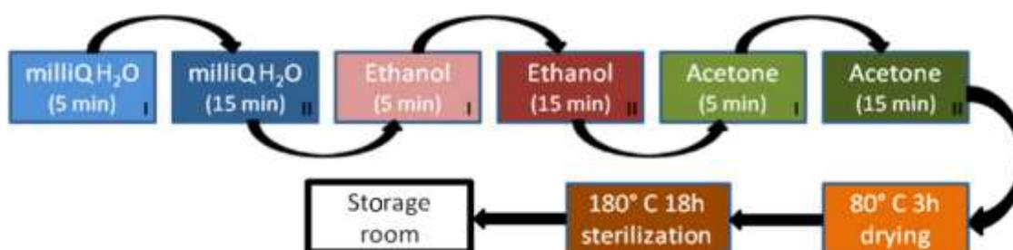
**Figure 1.** Scheme of the cleaning procedure for sample holders. All passages are made in sonicating baths with 1 lt solvent each. This volume is suitable for 10 open sample holders. Each second run can be done by using the solvent of bath II to fill bath I, while using fresh solvent for the new bath II. All operations are made in glove box.
