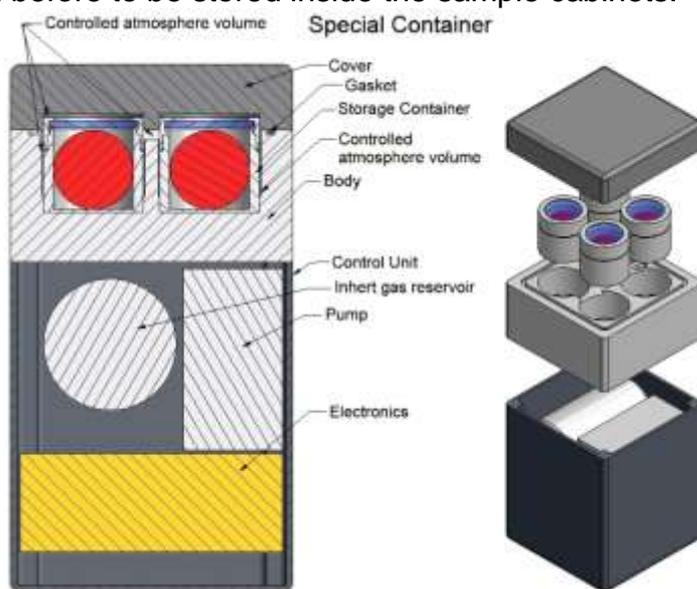
**Figure 3.** Special Container (courtesy Kayser Italia).
