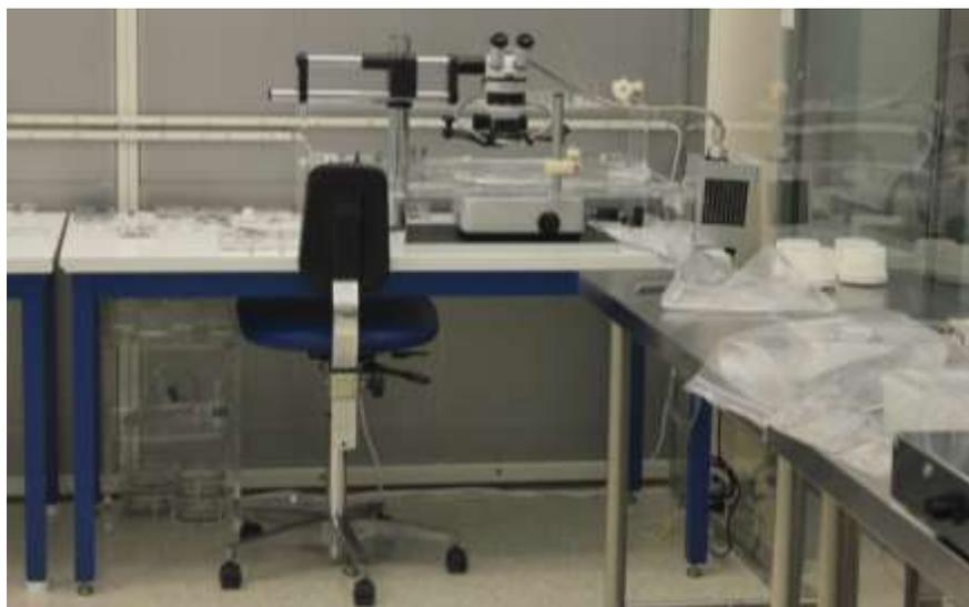
Fig. 12: Micromanipulator under a binocular microscope in the Cosmic Dust Laboratory.
