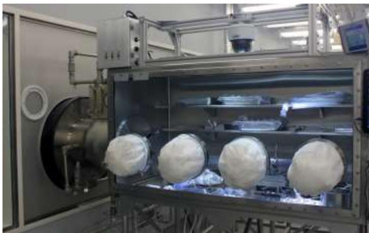
Fig. 5: A typical stainless steel glove box from the Lunar Laboratory (note the camera on top).
