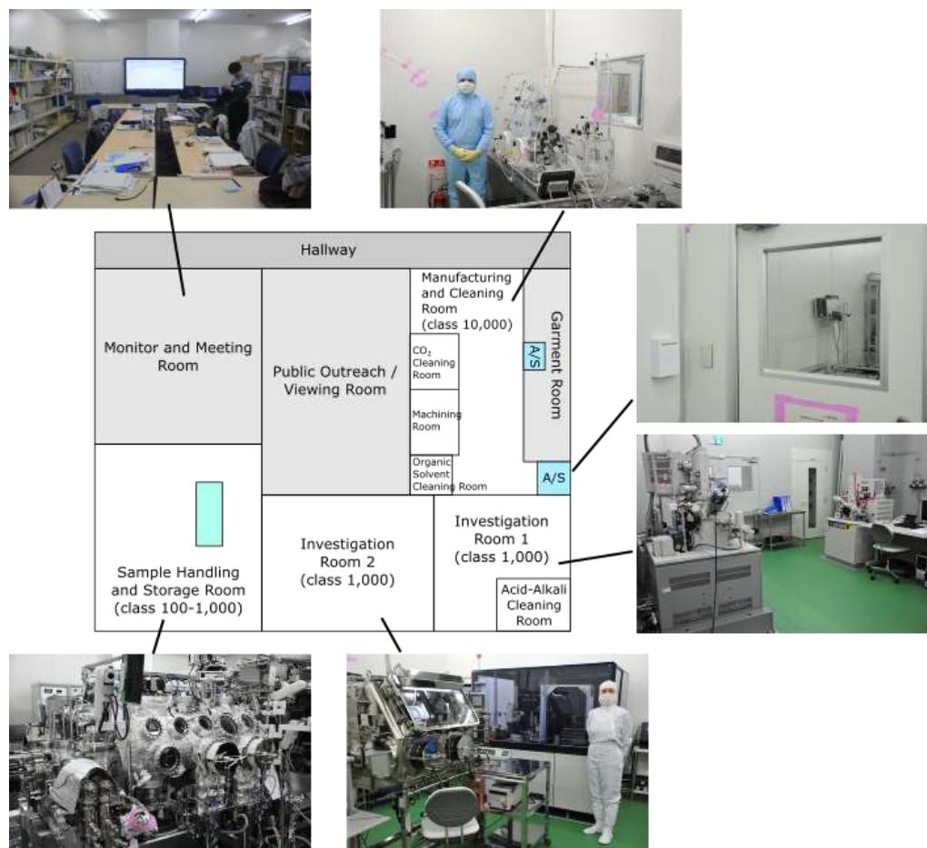
Fig. 1: A schematic viewgraph of the PMSCE/JAXA. Pictures showing (from top, clockwise): (i) the Monitor and Meeting room, (ii) Ludovic Ferrière inside of the Manufacturing and Cleaning Room, wearing a class 10,000 gown, (iii) the air shower between the Garment room and the cleaner part of the complex, (iv) the Investigation room 1, (v) Aurore Hutzler in the Investigation room 2, wearing a class 1,000 gown, and (vi) the clean chambers (used for handling and storage of the samples).
