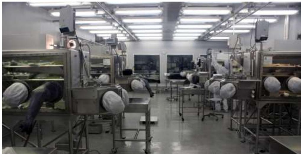
Fig. 3: Overview of the large curation room of the Lunar Sample Laboratory with several of the glove boxes.
