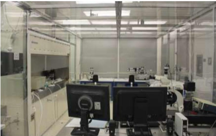
Fig. 11: Overview of the Cosmic Dust curation and preliminary examination room. It is equipped with optical and binocular microscopes; note on the left side the fume hood with ultrapure water system.
