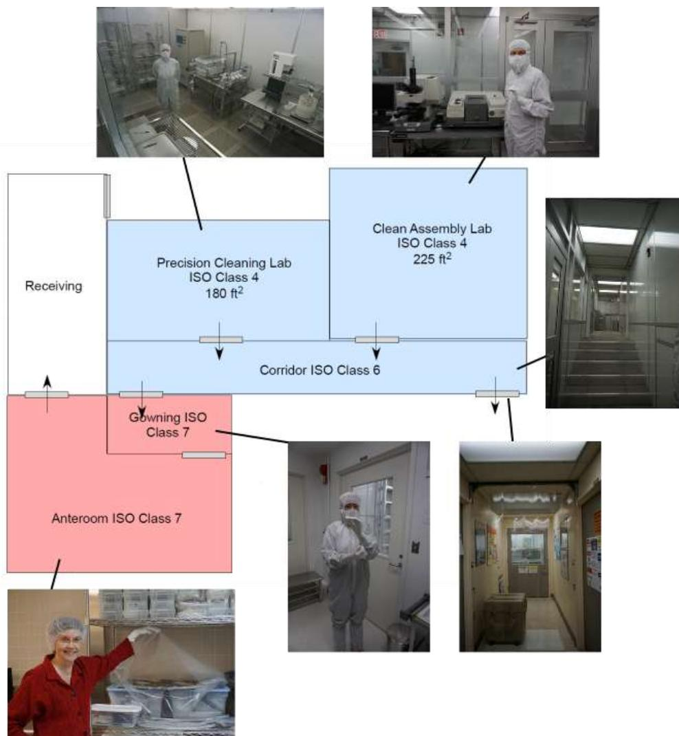
Fig. 6: Schematic viewgraph of the clean rooms of the Genesis Facility. Pictures showing (from top, clockwise): (i) Aurore Hutzler in the Precision Cleaning Lab, (ii) Judith Allton in the Clean Assembly Lab, in front of a FT-IR, (iii) the corridor in the cleaner part of the lab, (iv) the emergency exit from outside, (v) Aurore Hutzler in the garment room, adjusting an ISO 4 gown, and (vi) Judith Allton in the Anteroom, wearing only minimal protection.
