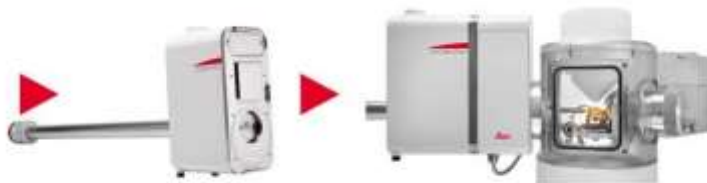
Fig. 12. Connection of the VCT to the dock installed on an instrument. (c) Leica.
