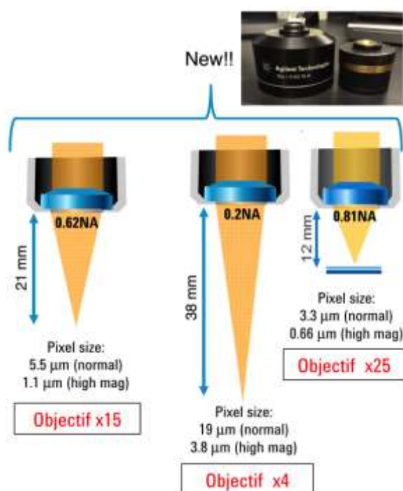
Fig. 4. Objective lenses available on the Cary IR microscope ((c) Agilent)
