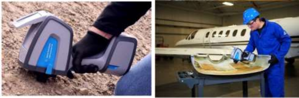
Fig. 1 Example of Handheld Topscan 4300 in the field (left) or for control of material quality (right). (c) Agilent.
